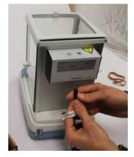
**10.** Attach the top frame and remove the elastic band.**11.** Connect the ioniser to the power supply.
