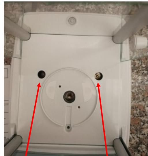
SCREW FOR CORNER LOAD REGULATION
